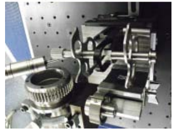
These photos show an example of a part that Gary Smith says the staff at GMI could not have attempted to machine without an advanced, ultra-precise CMM. The part is a spline rotor, which is key to the operation of a critical-function material feed system. The customer only provided a solid model (STEP file) and nominal dimensions. No conventional manufacturing drawings were available. Driven from the STEP files, Mitutoyo's CAD/CAM systems drove the part through CNC operations to completion.
