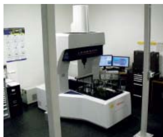
Mitutoyo Legex 574 CNC CMM as installed in the metrology laboratory at Gear Manufacturing Inc.
