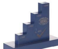
A stair step gage to test E_{UZ}
