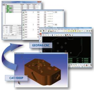
The nominal values are captured directly from the CAD model and tolerance values can be applied to various groups of size and location in the position GEOPAK-CNC part program.
