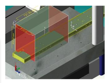
The CMM System Manager allows you create a virtual representation of your CMM for simulation. New Mitutoyo models or legacy models such as FN series and BHN series machines can be selecting based on machine stroke. If you have multiple machines they can also be added for simulation or part placement purposes. CAD models can be placed and compared to the true working volume of the machine and indexing probe swivel access.
