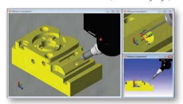
CAT1000P eliminates the time consuming task of data input from paper prints allowing your CMM to work in a paperless environment or by MBD (Model Based Definition).
